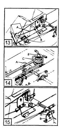
Remove the cap screw attaching the mower deck hanger to the front pivoting lift arm.
