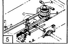
Slip the belt between idler pulley and belt guide tab of idler plate. Loosen (DO NOT remove) the cap screw securing the idler pulley to the idler plate.
