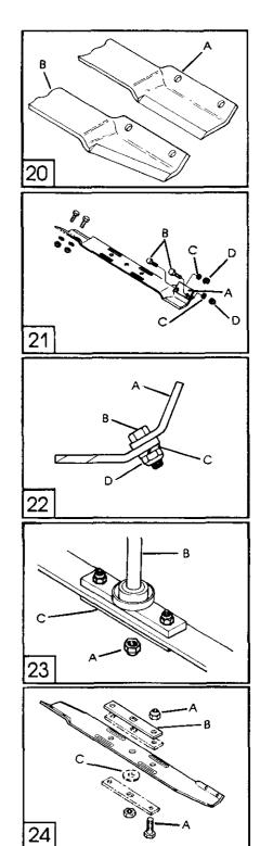
Install **both** blade support bars onto spindle shaft, then install new, "FLAT BLADE" below them.
